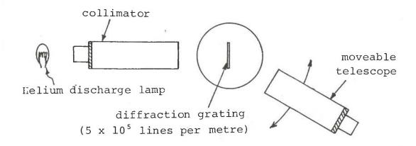
A student uses a spectrometer to find the wavelength of the prominent lines in the emission spectrum of helium. He measures the angle (20) between the two first order maxima for each spectral line. His results are tabulated below. Calculate the wavelength of each line. Write your answer in the appropriate column in the table below.
