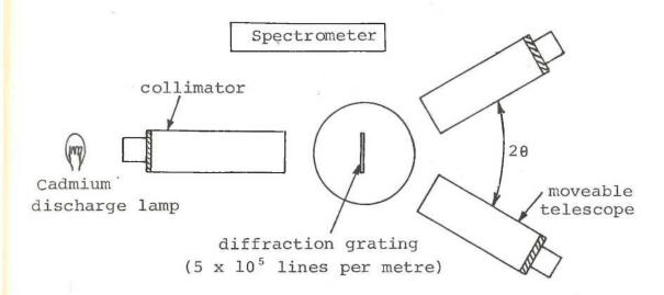
A student studies the emission spectrum of Cadmium using a spectrometer and diffraction grating as shown. For each spectral line she measures the angle 20. Find 20 for the lines listed below and write your answers in the appropriate column in the table.
